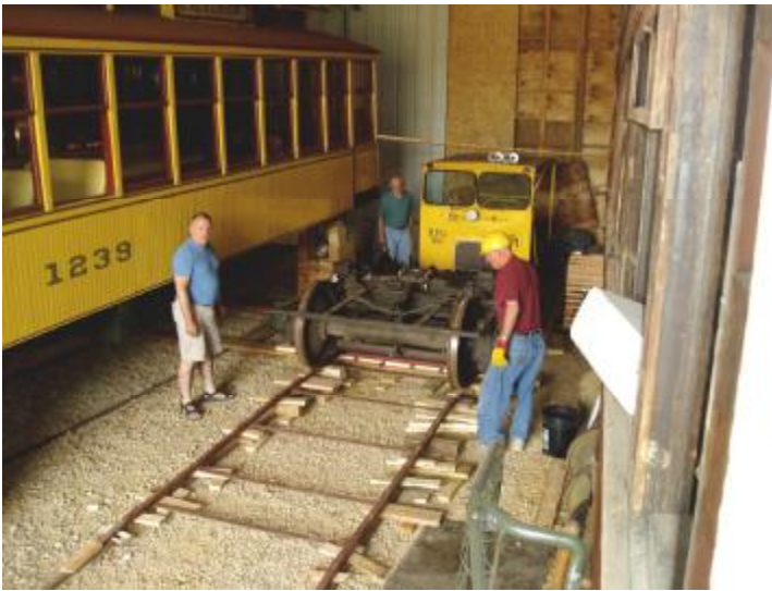
(Above Left) Putting No. 1239 back together entailed getting the two axles back in the trucks and lowering the motors onto the axles. The trucks were then put back under No. 1239 and the motor leads hooked up. The front truck went under the car easy enough but the rear truck had to be slid sideways to get where it needed to go. Here we see the rear truck on it's transfer table and (left to right) Bill Graham, Bob Johnson and Ken Albrecht considering the next move of that rear truck that needs to slide to the left under No. 1239. (John Prestholdt photo)
