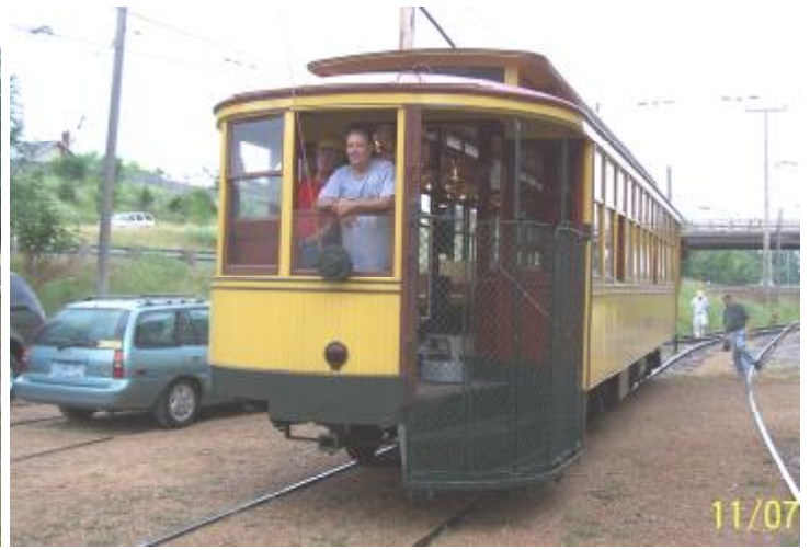
(Above Left) No. 1239 made it to the main line and we're now ready to test the car. The car was driven slowly the length of the line with some of the guys walking along side to check the wheel gauge and to look for other problems. (Above Right) That's Jim Willmore ready to put No. 1239 back into the barn after the test run. He looks happy and rightly so. Jim, and the others involved in the project are justifiably pleased with their work. Those others include Jerry Olsen, Phil Settergren, Ken Albrecht, Tom Fairbairn, Bob Johnson, Bill Graham, Dick Stoner, and John Prestholdt.
