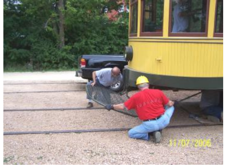
(Above Left) Putting No. 1239 back together entailed getting the two axles back in the trucks and lowering the motors onto the axles. The trucks were then put back under No. 1239 and the motor leads hooked up. The front truck went under the car easy enough but the rear truck had to be slid sideways to get where it needed to go. Here we see the rear truck on it's transfer table and (left to right) Bill Graham, Bob Johnson and Ken Albrecht considering the next move of that rear truck that needs to slide to the left under No. 1239. (John Prestholdt photo)
