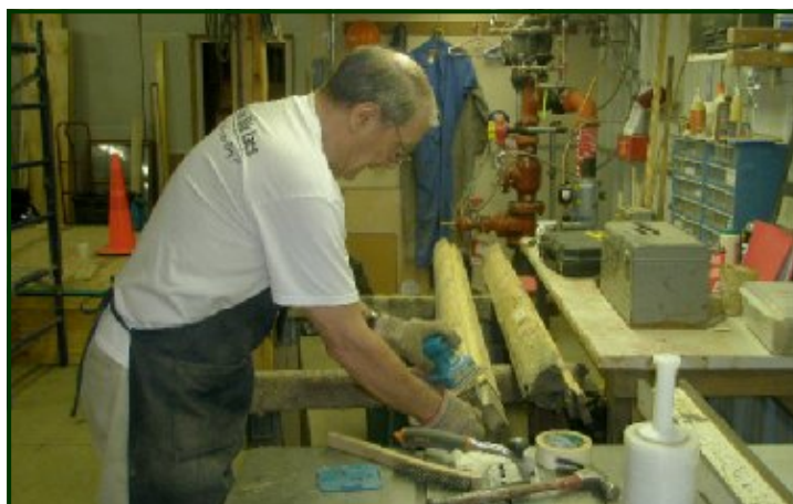
Here's George Ittner refinishing a vestibule end post.
